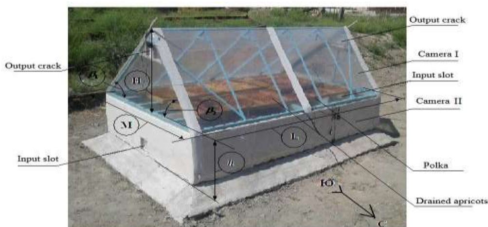
Fig. 1. Experimental direct type solar dryer.
